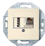
RJ45/TAE combination socket For the connection of a telephone and an analogue or digital terminal unit via the 8-pole RJ45 socket. To be completed with central plate art. no. 2928 .., 2978 .., 2938 .., 2979 .. or intermediate ring art. no. 5171 .., 5160 .., 5181 .. or intermediate ring with hinged lid for telecommunication connection sockets art. no. 5174 .., 5182 ..
