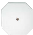
Cable exit for extension telephone sockets VDo 4 art. no. 4653 04 or general cable outlet up to Ø10 mm max. With central screw for fixing to the connector socket. Without claws for screw fixing.
